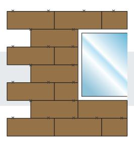
Wall ties of the correct type should be installed where required, and be suitable for their intended use and location.
