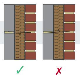
Where extra ties are required, e.g. at the side of openings, DriTherm® Cavity Slabs should be cut and fitted carefully around them. When off-cuts of DriTherm® Cavity Slab are needed, the batts can be cut with a long bladed knife or
