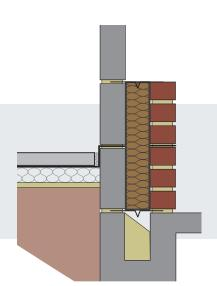
DriTherm® Cavity Slabs can be used in situations where they bridge the DPC in walls. Tests by the British Board of Agrément confirm that DriTherm® Cavity Slabs will not transmit water to the inner leaf, nor will they transmit moisture by capillary action across the cavity or from below damp proof course level provided they are installed correctly.
