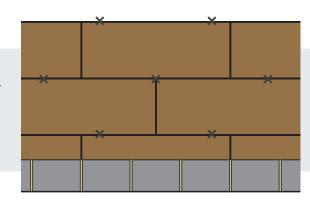
Where cavity insulation batts or slabs start below DPC level, the vertical and horizontal spacing of wall ties should be compatible with the spacing to be used above DPC level.
