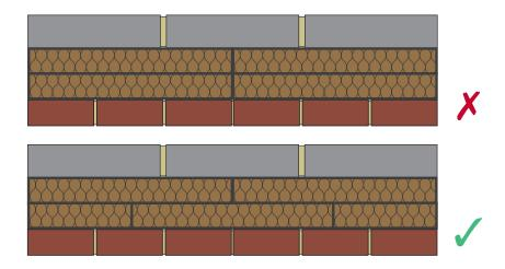
It is recommended that mineral wool batts with a thickness of 75mm or less are bent around corners to ensure that no gaps are left between batts, into which mortar could fall. Otherwise ensure joints are closely butted.
