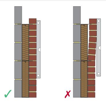
Knauf Insulation and NHBC recommend a cavity of uniform thickness is maintained throughout the construction and therefore we do not recommend rough stone to be used. Where natural stone is specified, we recommend the stone is cut to face to ensure the resultant cavity is uniform and parallel and stone is in accordance with this recommendation or alternatively a backing block is used in the outer leaf.
