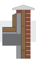
At eaves, cavity insulation should terminate at the top of the wall to meet the insulation at ceiling level. This ensures continuity between the wall and roof insulation and prevents any unwanted heat loss at the junction.
