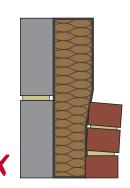
In fully filled applications, the type of insulation, its thickness and the wall construction should be suitable for the exposure of the building. (See Page 19).
