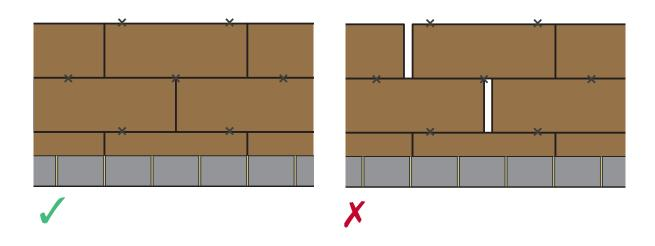
Any cutting and fitting should be neatly done, so not to distort the layers of glass wool which could compromise the material's performance.
